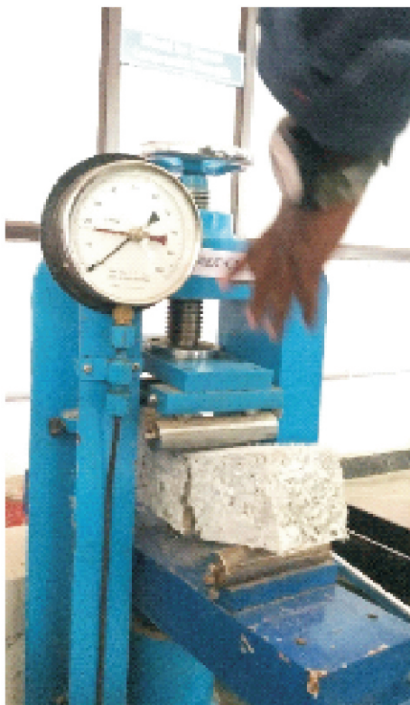
Figure 9. Concrete Prism Specimen after Flexure Testing
