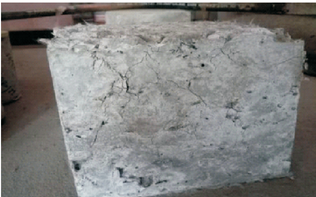
Figure 5. Cube Specimen After Compression Testing
