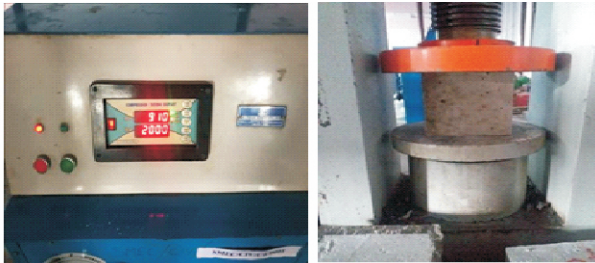
Figure 4. Compression Testing for Cube specimens
