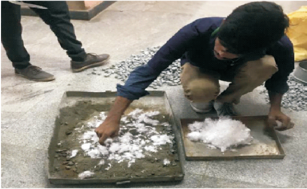
Figure 2. Mixing of Fiber Reinforced Concrete
